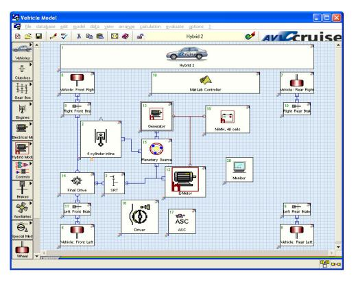
Depending on the calculation task and the desired accuracy of the results, the complexity (modeling depth) of the vehicle models can be increased from simple to complex continuously in a very efficient way.
