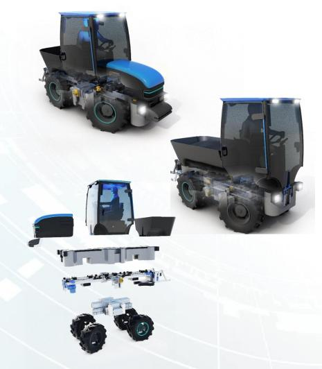
Apart from the conventional small tractor structure, AVL developed a flexible, cost-efficient and high-performing solution for small volumes and small-size tractors. The concept is not limited to one type of machine. It combines the cost-driving components, such as the electric drives, batteries or power electronics in a base chassis, which can be used for a tractor or a harvesting or maintenance machine on the same power level.
