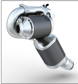
Figure 2: Final EAS design after CFD optimization
