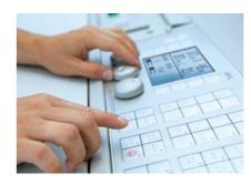
The operating panel allows you to operate the testbed using push-buttons and incremental pulse wheels • User-friendly handling through ergonomic design of operating
