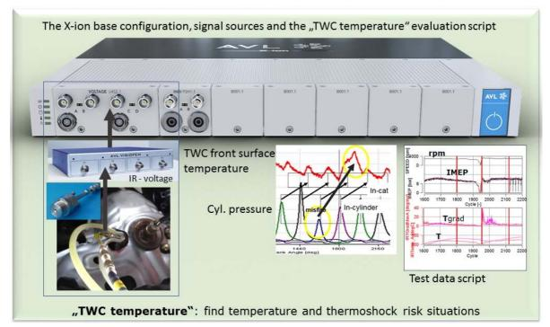
Sensors, instrumentation and signal examples
