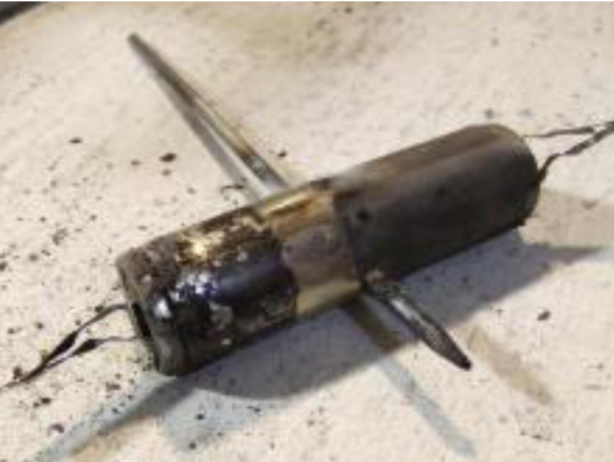
Nail Penetration according to GB/T 31485-2015
