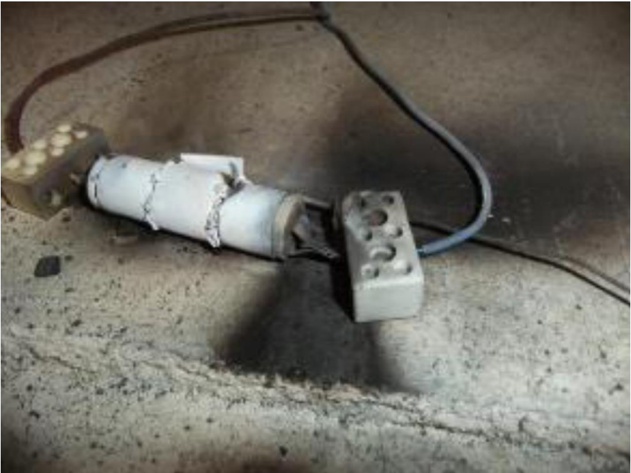
Thermal Stability according to SAE J2462
