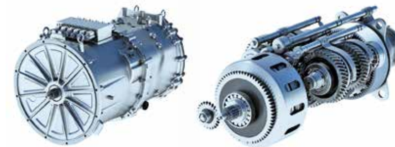
AVL DCT concept for Trucks / Bus applications
