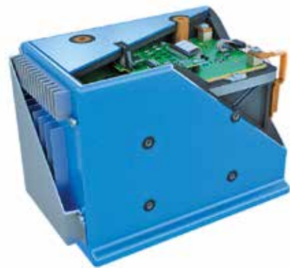
Low-cost 48V battery technology demonstrator
