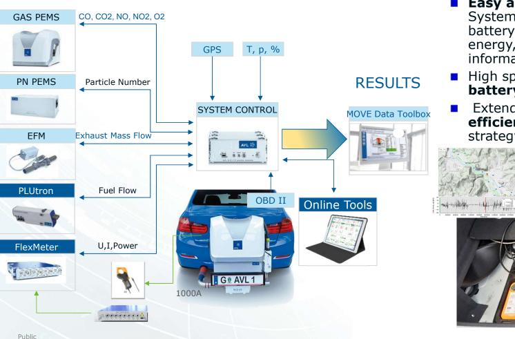
Easy add-on of hybrid key figures into System Control (real fuel consumption, battery state of charge, Recuperated energy, charging modes, HCU information)
