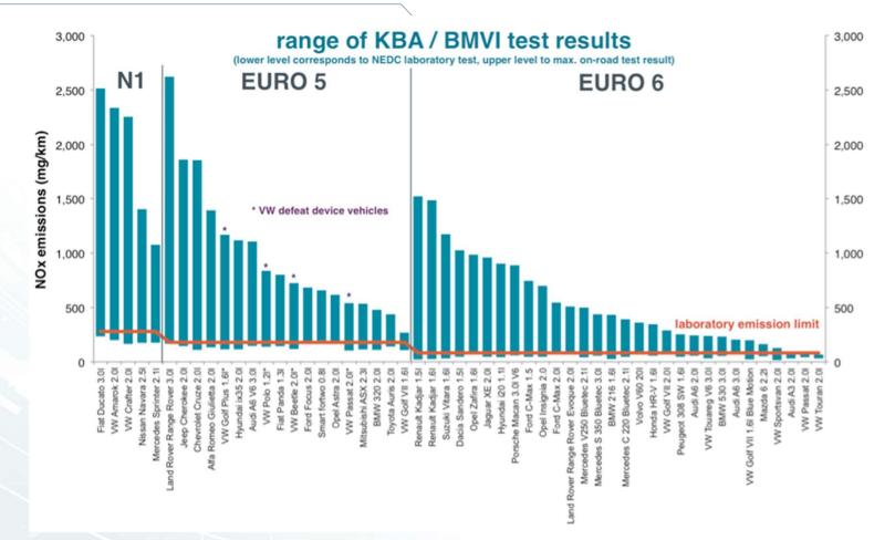
Source: Overview of the laboratory and on-road test results of the vehicle testing program by the German Ministry for Transport
