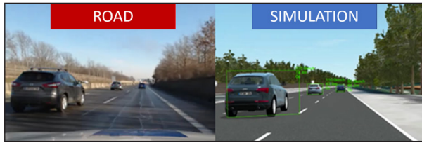
Fig. 9: Digital twin: Matched scenarios in vehicle road test (left) and vehicle simulation (right) to check correlation of real and virtual domain, based on matching physical signals and objective assessment.
