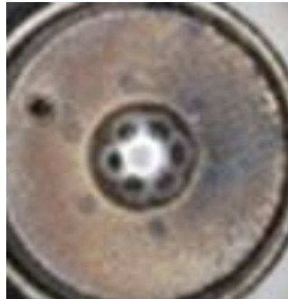
coked injector tip
