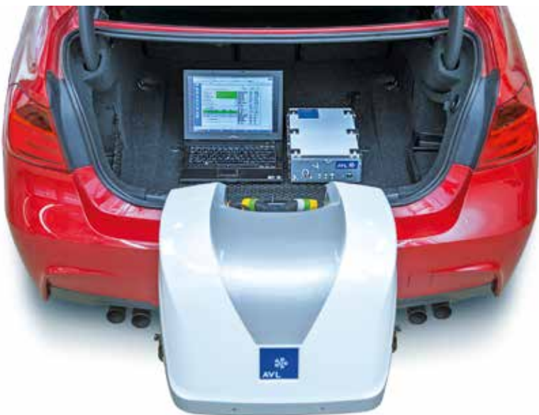
Outside installation on a tow bar. Trunk: System Control with Notebook PC
