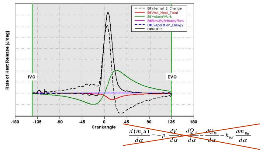
dQ<sub>f</sub>: heat release by combustion after fuel injection
