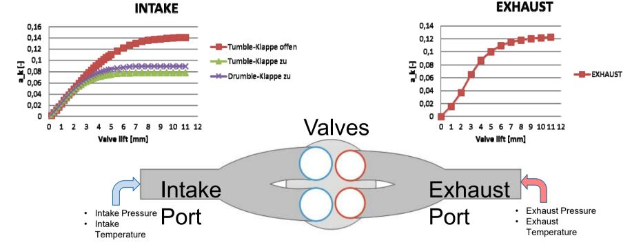
For calculation of gas-exchange **Port** and **Valve Data** for Intake and Exhaust are needed:
