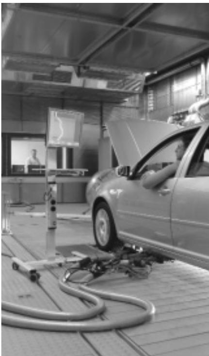
Since introducing AVL-Drive as objective vehicle driveability assessment tool the entire system has been improved considerably. Nowadays, more driveability measurements are done on the roller chassis dynamometer to perform basic Engine and Transmission application tasks and fine adjustments much quicker with improved reproduction quality.
