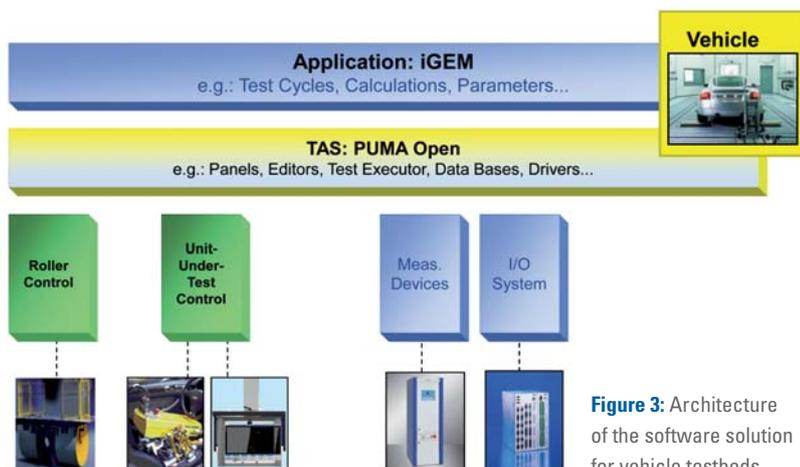
Figure 3: Architecture of the software solution for vehicle testbeds
