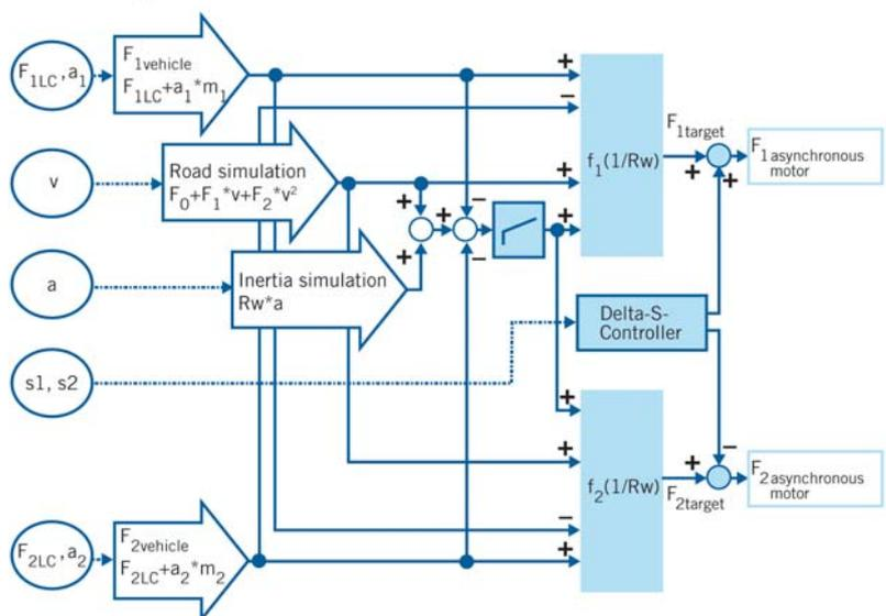
Figure 4: Controller configuration for single and twin axle test beds
