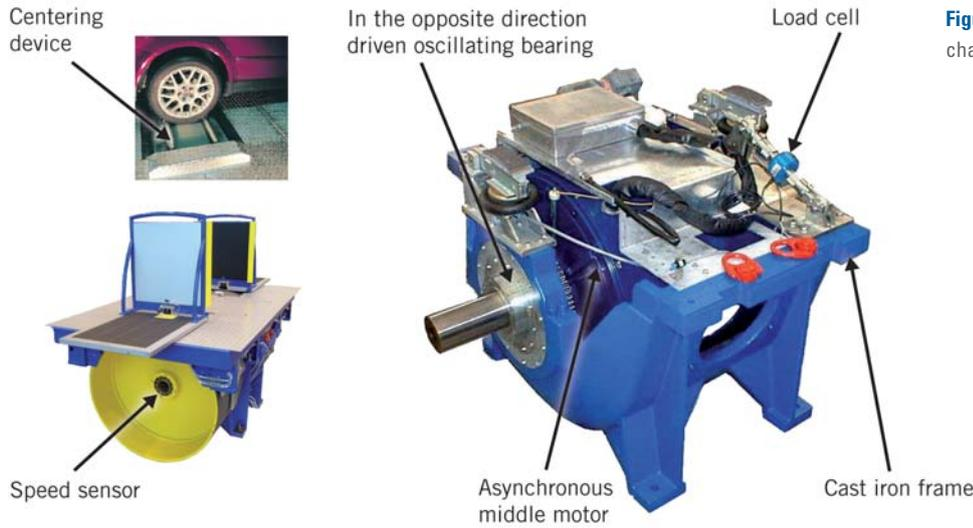
Figure 3: Hardware components of the chassis dynamometer
