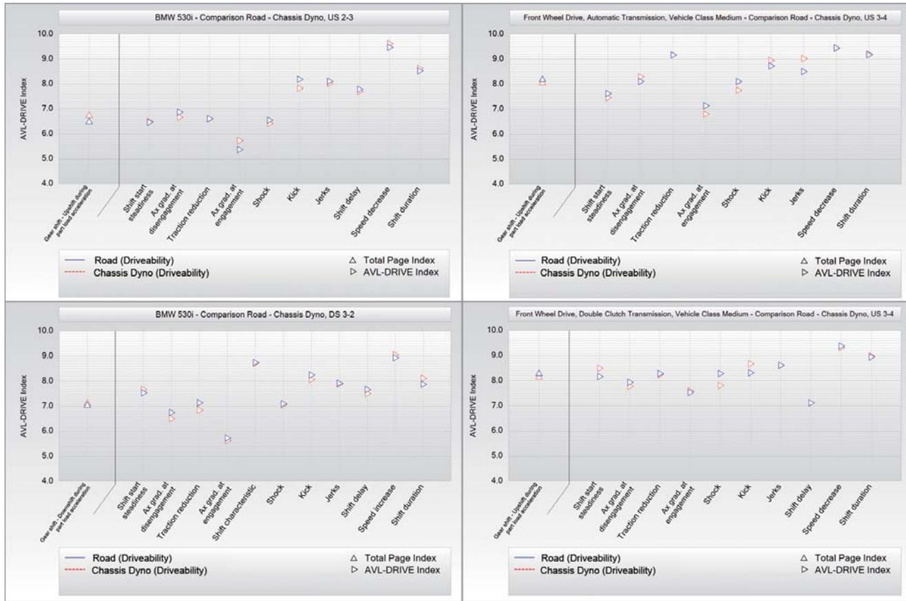
Figure 6: Comparison of driveability ratings for shift quality between road and chassis dyno
