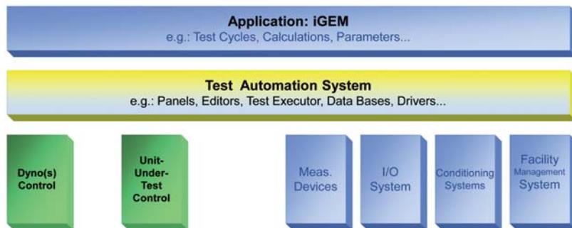
Figure 2: The architecture of a common automation platform
