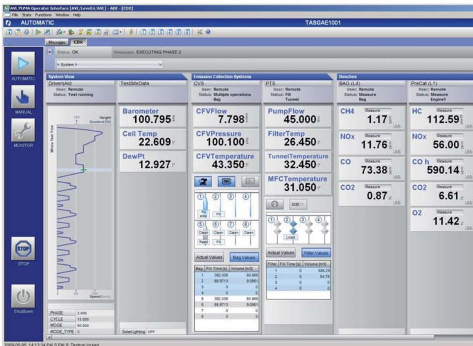
**Figure 4:** The PUMA Open automation system with iGEM Vehicle for vehicle emission certification
