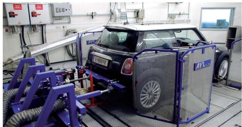
**Figure 5:** System layout, test vehicle on the high dynamic chassis dynamometer
