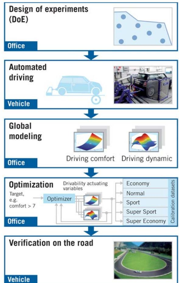
Figure 2: General work process of the model-based calibration of driveability
