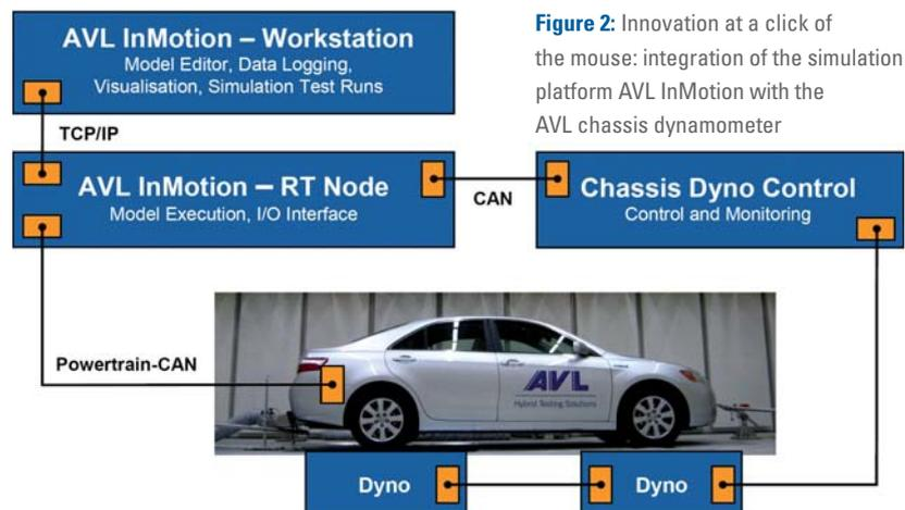
**Figure 2:** Innovation at a click of the mouse: integration of the simulation platform AVL InMotion with the AVL chassis dynamometer
