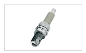
The ZI31 is a spark-plug with integrated pressure sensor. The M12 design has very small eccentricity of the center electrode. This and the high sensitivity of the sensor elements combined with the high stiffness of the spark plug body guarantees excellent measurement performance. The insulator of the spark-plug is developed and manufactured by Bosch. The sensor can be equipped with SDC to make it ready for SDM Sensor Data Management.
