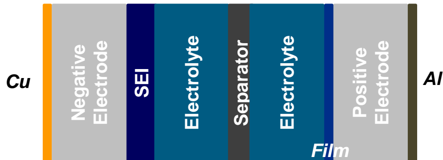
Example: Liquid electrolyte lithium battery
