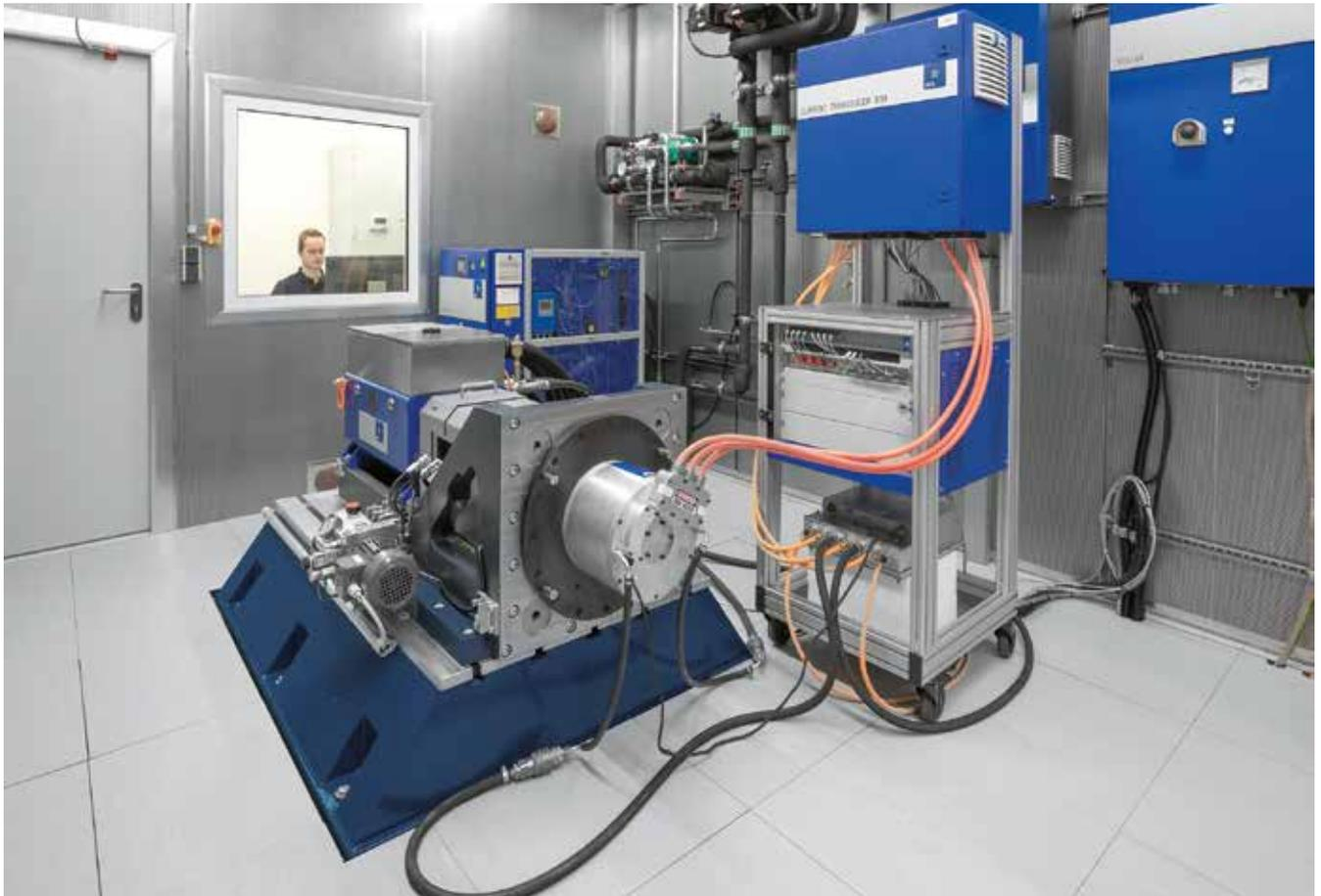
AVL E-Drive Testsystem in Modularbauweise.
