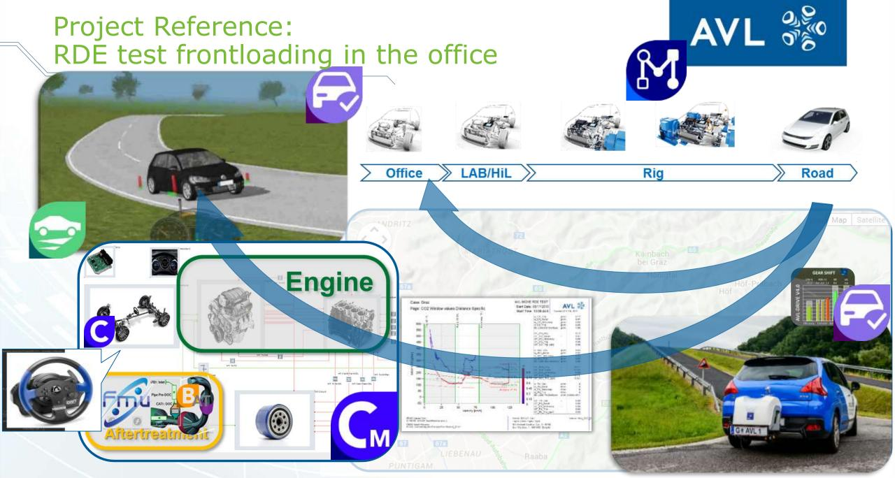
Customer Reference: Real Driving Emission Testing Environment on Engine Testbed
