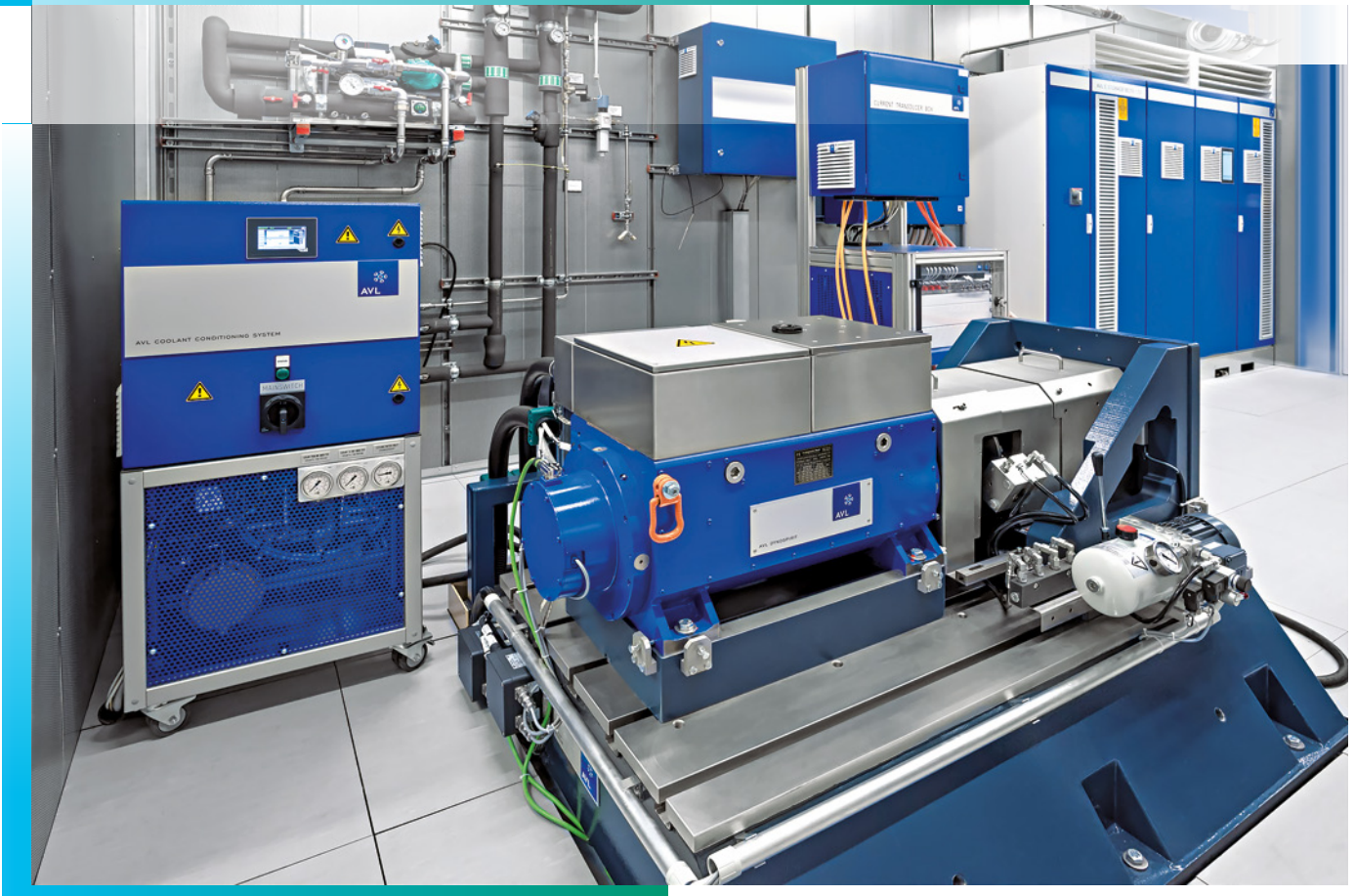
AVL E-Motor T5™ consisting of a dynamometer, battery emulator, conditioning systems and e-power analyzer.
