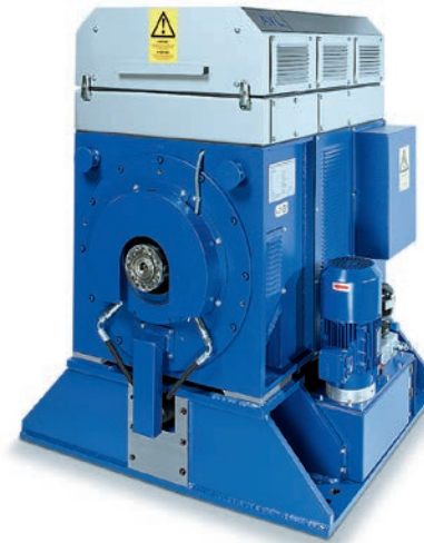
Highly precise, pendulum-mounted, robust AC drive system with a state-of-the-art 4Q-IGBT converter for speed and torque-controlled operation. A real-time torque calculator also provides the shaft torque of the machine in addition to the electric torque (air-gap torque).
