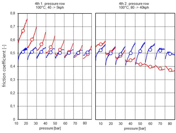
**Friction coefficient: GCI disc + GCI brake pad**
