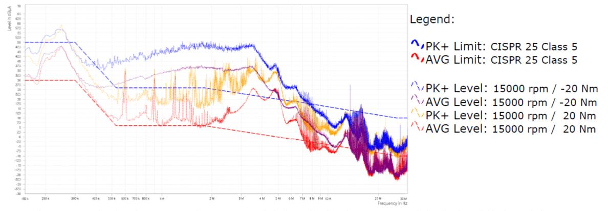
Note: the measurements have been done in a pre-compliance environment, the background level interference emissions are higher than demanded by the standards
