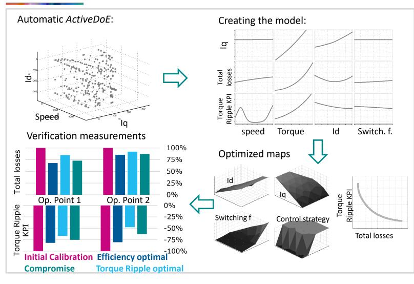
In a model-based way by using active-DOE an e-drive was optimized on a testbed
