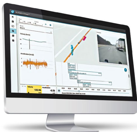
◀ The Big Data and Analytics Platform's scenario viewer provides a synchronized view of video, object, time-series and map data for a clear visual interpretation of the test drive.
