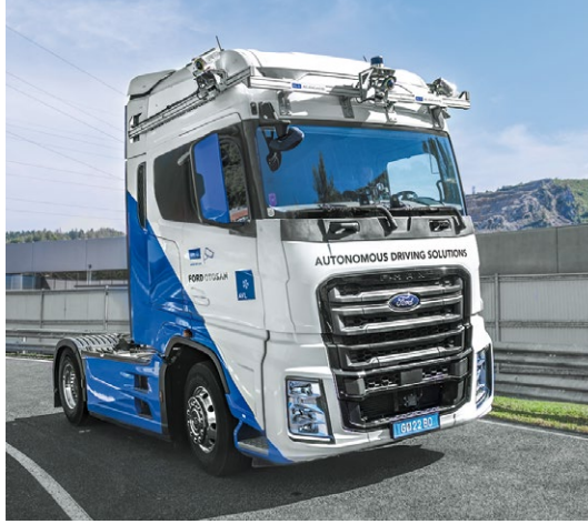
▲ The AVL Ground Truth System collects a highly precise reference of the traffic environment.
