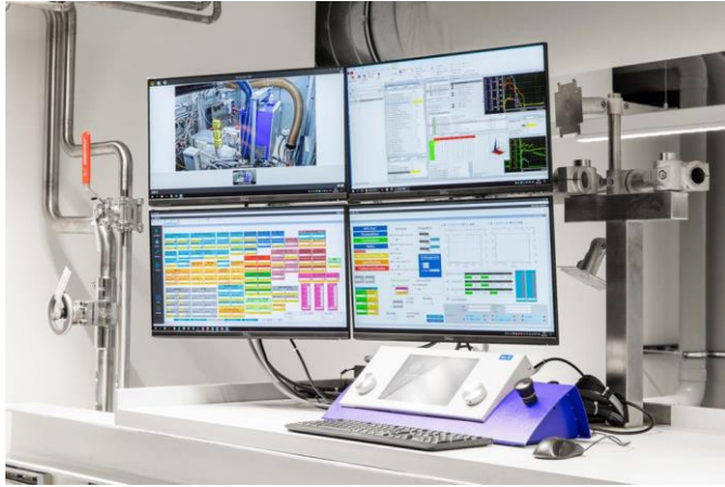
Test bed automation & control system AVL PUMA2™ for fuelcell
