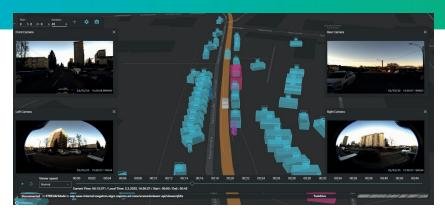
For visualization of your recorded data the **Scenario Viewer** can be used to show detected objects, lines, camera images, etc.
