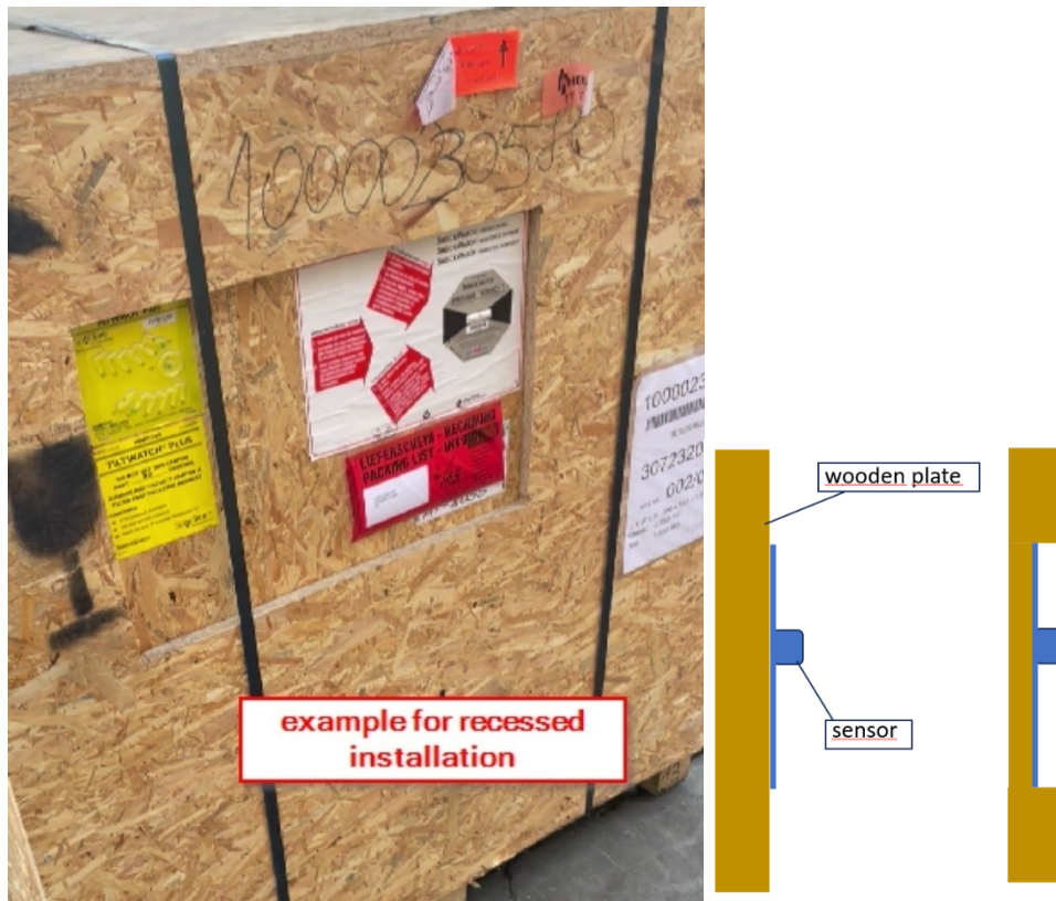
Figure 13: Specification for the installation of the indicators
