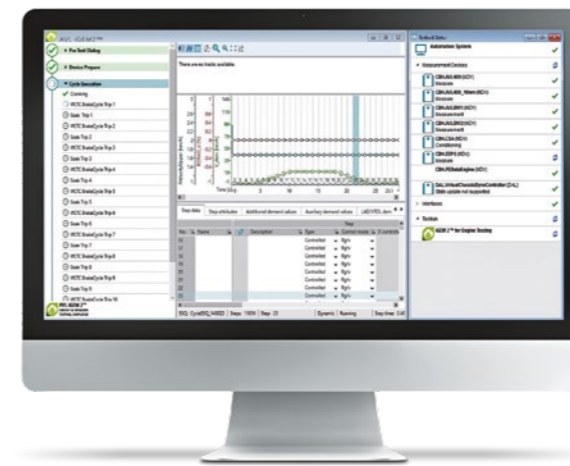
▲ The iGEM 2 test automation system guides you through the entire brake test procedure, including pre-test dialog, test preparation and the test run itself. The test cycle is run automatically in an unmanned mode.
