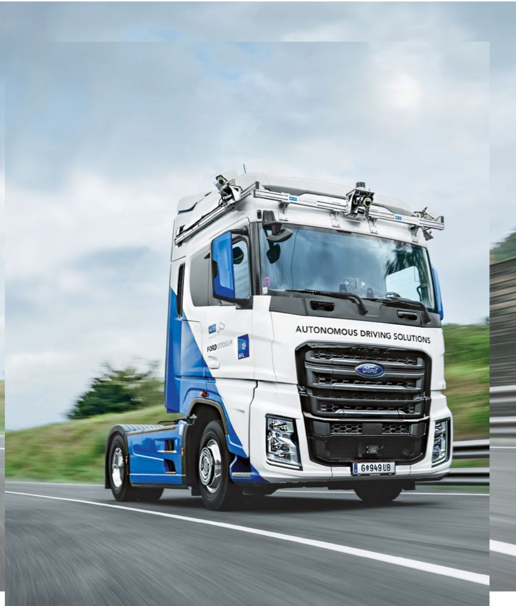
▲ Truck with Dynamic Ground Truth System
